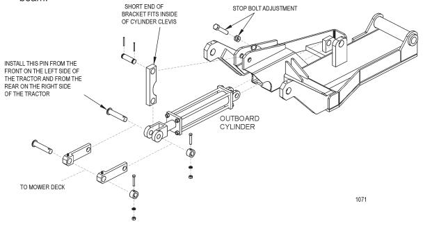
Slide other end of pivot arm with short distance between the cut-out and the end of the pivot arm, into the cylinder clevis. Next, line up the holes of the left and right lift linkage arms outside of the cylinder clevis holes. Connect with linkage pin, shims (as required), boss, cap-screw, lock-washer and hex nut as shown.
